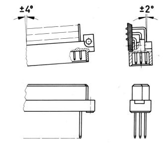
To ensure reliable connections and prevent unnecessary damage, please refer to the application data diagrams. These recommendations are set out in IEC 60603-2.
