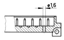
To avoid cross-plugging of adjacent connectors a coding system is required.
