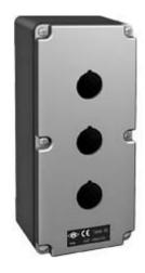
Box for control devices and signals, AC series, M25 cable entry, 3 holes for unit Ø 22 mm, external dimensions 92x205x86 mm
