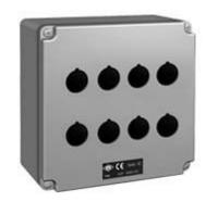
Box for control devices and signals, AC series, M25 cable entry, 8 holes for unit Ø 22 mm, external dimensions 152x152x86 mm
