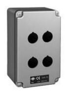
Box for control devices and signals, AC series, without cable entry, 4 holes for unit Ø 22 mm, external dimensions 92x152x86 mm
