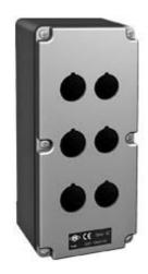
Box for control devices and signals, AC series, without cable entry, 6 holes for unit Ø 22 mm, external dimensions 92x205x86 mm
