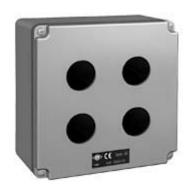
Box for control devices and signals, AC series, without cable entry, 4 holes for unit Ø 30 mm, external dimensions 152x152x86 mm
