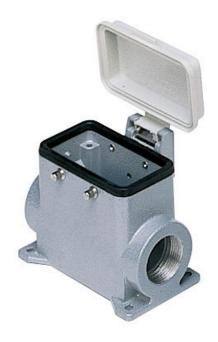
Surface mounting housing, C-TYPE series, with 4 pegs, M32 cable entry, size "57.27", high construction, with plastic cover
