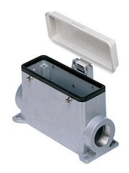
Surface mounting housing, C-TYPE series, with 4 pegs, M40 x 2 cable entry, size "104.27", high construction, with plastic cover
