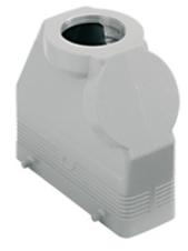
Hood, C-TYPE series, with 4 pegs, M50 top cable entry, size "104.27", high construction, inclined
