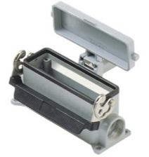
Surface mounting housing, 830V series, with 1 lever, M40 x 2 cable entry, size "104.27", high construction, with metal cover
