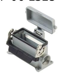
Surface mounting housing, 830V series, with 1 lever, M25 cable entry, size "77.27", with metal cover
