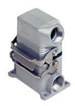
Complete connector, CNZ series, composed of 2 screw terminal connection inserts with 6 poles + PE, and surface mounting housing with 1 lever and hood with side cable entry
