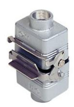
Complete connector, CNZ series, composed of 2 screw terminal connection inserts with 6 poles + PE, and hoods with top cable entry and closing with 1 lever
