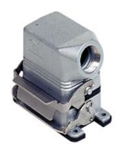
Complete connector, CNZ series, composed of 2 screw terminal connection inserts with 24 poles + PE, and bulkhead mounting housing with 1 lever and hood with side cable entry
