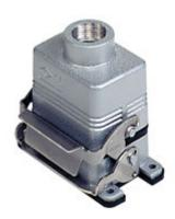
Complete connector, CNZ series, composed of 2 screw terminal connection inserts with 24 poles + PE, and bulkhead mounting housing with 1 lever and hood with top cable entry
