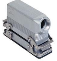
Complete connector, CNZ series, composed of 2 screw terminal connection inserts with 10 poles + PE, and bulkhead mounting housing with 2 levers and hood with side cable entry
