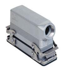
Complete connector, CNZ series, composed of 2 screw terminal connection inserts with 16 poles + PE, and bulkhead mounting housing with 2 levers and hood with side cable entry
