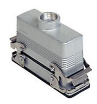
Complete connector, CNZ series, composed of 2 screw terminal connection inserts with 24 poles + PE, and bulkhead mounting housing with 2 levers and hood with top cable entry
