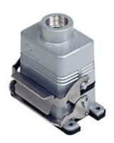
Complete connector, CSZ series, composed of 2 spring terminal connection inserts with 6 poles + PE, and bulkhead mounting housing with 1 lever and hood with top cable entry
