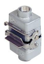
Complete connector, CSZ series, composed of 2 spring terminal connection inserts with 6 poles + PE, and hoods with top cable entry and closing with 1 lever
