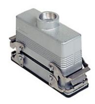
Complete connector, CSZ series, composed of 2 spring terminal connection inserts with 10 poles + PE, and bulkhead mounting housing with 2 levers and hood with top cable entry
