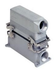
Complete connector, CSZ series, composed of 2 spring terminal connection inserts with 10 poles + PE, and surface mounting housing with 2 levers and hood with side cable entry
