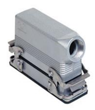
Complete connector, CSZ series, composed of 2 spring terminal connection inserts with 16 poles + PE, and bulkhead mounting housing with 2 levers and hood with side cable entry
