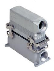
Complete connector, CSZ series, composed of 2 spring terminal connection inserts with 16 poles + PE, and surface mounting housing with 2 levers and hood with side cable entry
