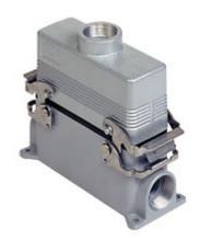
Complete connector, CSZ series, composed of 2 spring terminal connection inserts with 16 poles + PE, and surface mounting housing with 2 levers and hood with top cable entry
