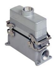
Complete connector, CSZ series, composed of 2 spring terminal connection inserts with 24 poles + PE, and surface mounting housing with 2 levers and hood with top cable entry
